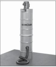
collector investment. The 50 micron polyfelt bag filter is easily laundered and replaced.
